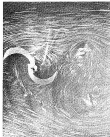
Fig. 19 A typical set of flow visualization pictures showing the presence of the central vortex filament
